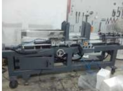
Fig.12. Assembly of Pinning Machine
